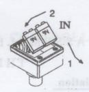
First insert the rear end of the battery and only then firmly push the front side of the battery into position.
